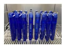
First of all, please leave the heat storage materials at intervals of 4 to 8 hours in anenvironment of 45°C (such as an incubator) and confirm that the material iscompletely liquid. Next, please stand for 1 hour in an environment of 36°C or 10~15 minutes at room temperature (20 ~25°C).
