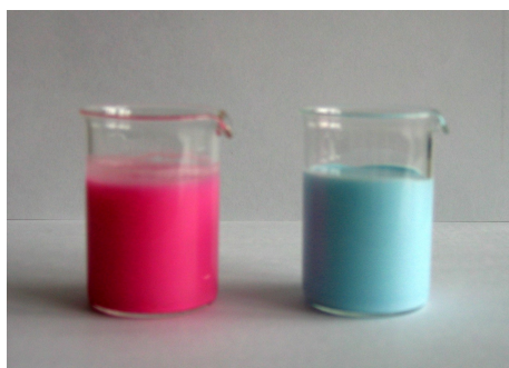
sicastar®-red and sicastar®-blue, suspension in water, particle size 1 µm, plain
