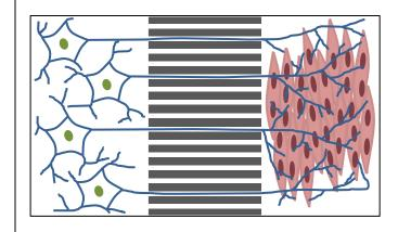
Fig. 1. Schematic representation of co-culturing motor neurons with muscle cells within Xona's devices and chips. Motor neurons grow in one compartment and extend their axons to innervate muscle cells cultured in the adjoining compartment. The microgroove barrier separates the two compartments and allows each compartment to be treated independently.
