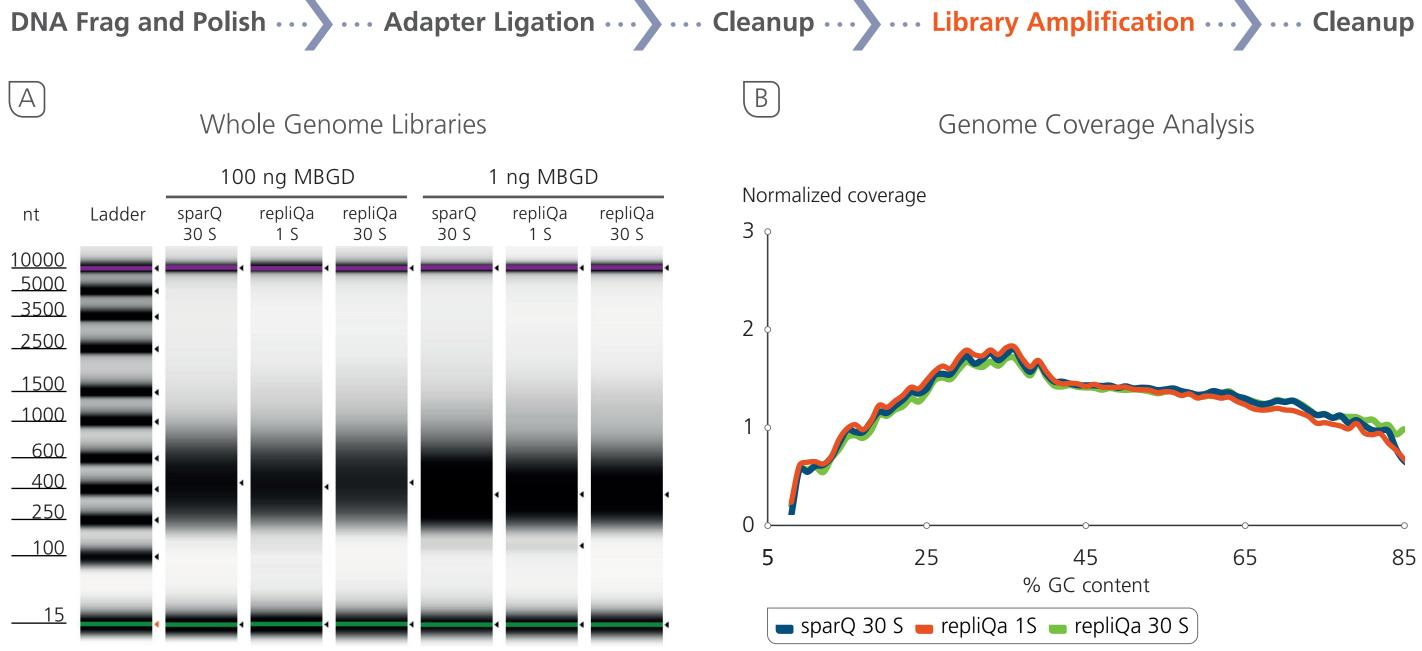
Figure 4 Whole genome library amplification. Whole genome libraries were prepared from mixed bacterial genomic DNA (MBGD) using sparQ DNA Frag & Library Prep Kit. Libraries were amplified with either sparQ HiFi PCR Master Mix with a standard 30 s extension time or repliQa HiFi ToughMix with either a 1 s or 30 s extension time. (A) TapeStation analysis of the prepared libraries. (B) Genomic coverage across 5 to 85% of GC content.
