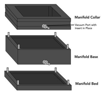
Diagram of EZ-Vac 96<sup>™</sup> Vacuum Manifold
