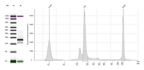
**Characterization of a completed control library**. Agilent TapeStation® 4150 D1000 electropherogram of a typical **Zymo-Seq<sup>TM</sup> miRNA Library** using 1  $\mu$ L of the included positive control (10 fmol of a random 21-mer) using 16 PCR cycles. 10 fmol of the control is approximately 67 pg/ $\mu$ L. **A1** is a molecular weight marker, and **B1** is the completed miRNA library.
