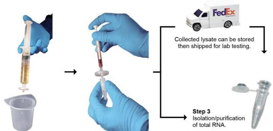
Make sure guidelines are followed to ensure the RNA isolation procedure is performed in an RNase-free environment.
