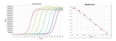
Reliable Standards for the Quantification of Human DNA: Human DNA Standards performed in duplicates 10-fold serial dilutions ranging from 20 ng to 20 fg.
