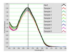
Pure and Reliable Recovery with the DCC®-5. Shown here is the recovery of 1 µg of 100 bp marker DNA eluted into 10 µl of water analyzed using a NanoDrop® spectrophotometer. The DNA Clean & Concentrator®-5 consistently recovers > 90 % of input DNA.
