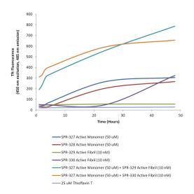
Thioflavin T is a fluorescent dye that binds to beta sheet-rich structures, such as those in tau fibrils. Upon binding, the emission spectrum of the dye experiences a red-shift, and increased fluorescence intensity. Thioflavin T emission curves show increased fluorescence (correlated to tau aggregation) in active tau K18/PL monomers (SPR-328) over time. Thioflavin T ex = 450 nm, em = 485 nm.
