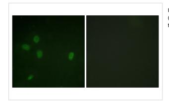
Immunofluorescence analysis of NIH/3T3 cells, using 53BP1 (Phospho-Ser25) antibody #12125. The picture on the right is treated with the synthesized peptide.
