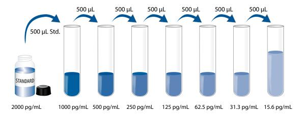
For Serum/Plasma Samples - Pipette 500  $\mu$ L of Calibrator Diluent RD6O into each tube. Use the stock solution to produce a dilution series (below). Mix each tube thoroughly before the next transfer. The undiluted standard serves as the high standard (2000 pg/mL). Calibrator Diluent RD6O serves as the zero standard (0 pg/mL).
