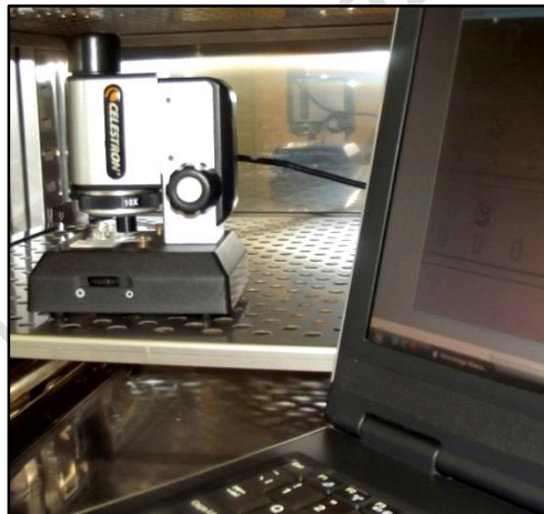
Fig.4. Time-lapse microscope in incubator
