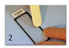
ii. Use the applicator stick provided to press along the adhesive areas to ensure a secure seal. Visually inspect the seal from underneath the microarray; inconsistent patterns in the black adhesive may indicate an insecure seal. Re-use the applicator stick if needed (Figure 2)
