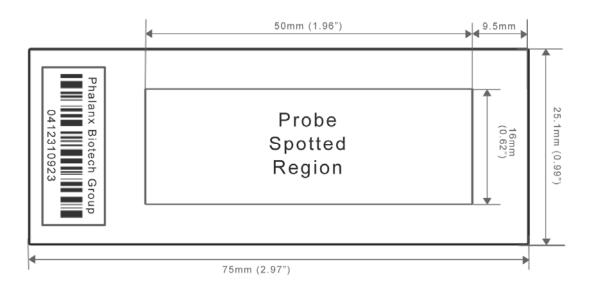
Figure 1: OneArray<sup>®</sup> Microarray Glass Slide with "Probe Printed Region Guide" Plastic Underlay.
