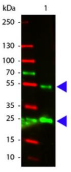
Western Blot of Atto 532 conjugated Rabbit anti-Goat IgG antibody. Lane 1: Goat IgG. Lane 2: none. Load: 50 ng per lane. Primary antibody: none. Secondary antibody: Atto 532 rabbit secondary antibody at 1:1000 for 60 min at RT. Block: MB-070 for 30 min at RT. Predicted/Observed size: 50 kDa, 25 kDa for Goat IgG. Other band(s): none.
