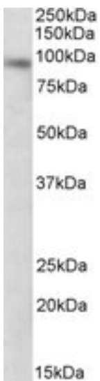
DTX3 antibody (0.3 ug/ml) staining of NIH3T3 lysate (35 ug protein in RIPA buffer). Primary incubation was 1 hour. Detected by chemiluminescence.
