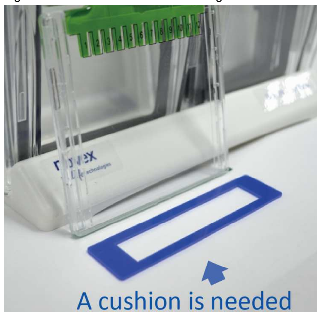
Figure 1. A cushion is needed to run a gel in Bolt™ Mini Gel Tank
