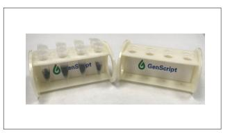
Holds: Eight standard 1.5- 2 mL micro-centrifuge tubes. Working volume : <2mL
