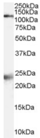
EB07341 (2 \mu g/ml) staining of Rat Brain lysate (35 \mu g protein in RIPA buffer). Primary incubation was 1 hour. Detected by chemiluminescence.
