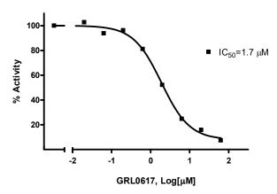
Inhibition of PLPro Deubiquitination activity by GRL0617, measured using the *Papain-like Protease Assay Kit: Deubiquitinase Activity (BPS Bioscience #79996).* Fluorescence intensity was measured using a Tecan fluorescent microplate reader. *Data shown is lot-specific.* For lot-specific information, please contact BPS Bioscience, Inc. at info@bpsbioscience.com
