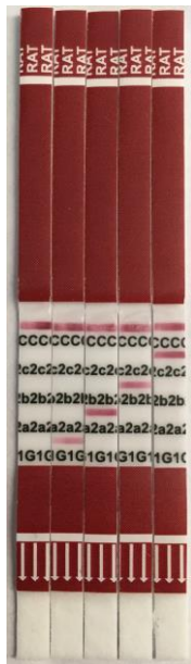
Figure 1 - Completed RIS1R-010 Lateral Flow Strips. Note that the red lines indicating a positive result are above the printing on the strip cover.
