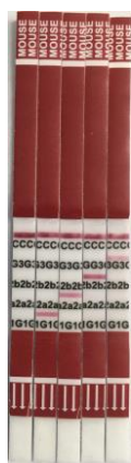
Figure 1 - Completed MIS1R-010 Lateral Flow Strips. Note that the red lines indicating a positive result are above the printing on the strip cover.
