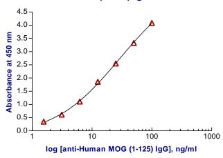
$Y=[(A-D)/(1+\{x/C\}^B)]+D, \underline{A}=-0.21 \underline{B}=0.787 \underline{C}=29.09 \underline{D}=5.687 R^2=0.999$
