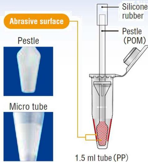
BioMasher II consists of a 1.5 mL microtube and a pestle. The sample and extraction buffer are placed in the tube, and ground to prepare the homogenate. The microtube and pestle are molded so that they fit without any space between them. The texture of the inner wall of the tube and the outer periphery of the tip of the pestle enhances the efficiency of the disruption of the sample.
