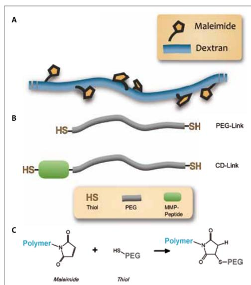
Figure 1: hydrogel components and cross-linking reaction. The maleimide dextran polymer is shown in A), crosslinker di-thiol-PEG with or without matrix metalloproteinase cleavage site in B), and the reaction scheme in C).
