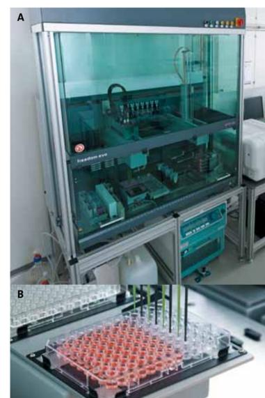
Figure 2: liquid handling robot. In A) the Freedom EVO robot is shown and B) a 96-well plate is filled with medium using fixed tips.
