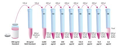
Figure 5. Preparation of the cortisol standards ASSAY PROTOCOL
