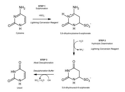
**Overview of Bisulfite Conversion**. Steps 1 and 2 occur during bisulfite conversion, while Step 3 is performed as the DNA is bound to the column matrix. For the reaction to proceed to completion, it is essential the DNA be fully denatured.
