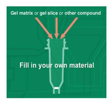
The MobiSpin Column "F" is designed for a wide variety of applications for nucleic acid and protein extraction and purification. When choosing the MobiSpin Column "F" for a particular application, a suitable resin must be selected and filled into the mini-column. For an appropriate resin selection, impurity versus sample size and the anticipated yield must be sonsidered.
