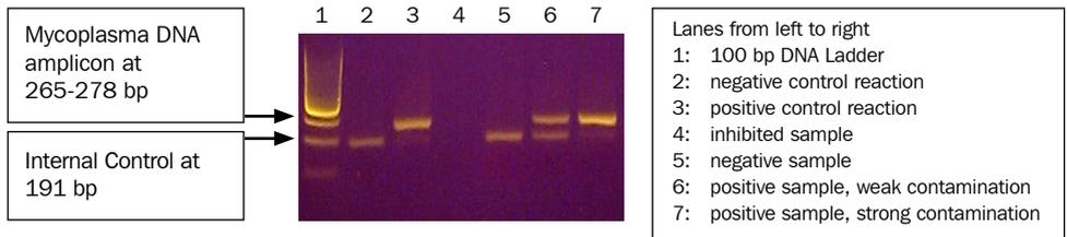
**Fig. 1:** A typical agarose gel image
