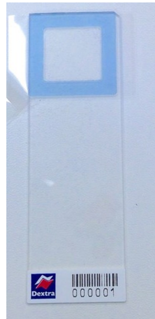
Figure 1b: Positioning of the top of the Gene Frame on the Glycan Array Kit slide.
