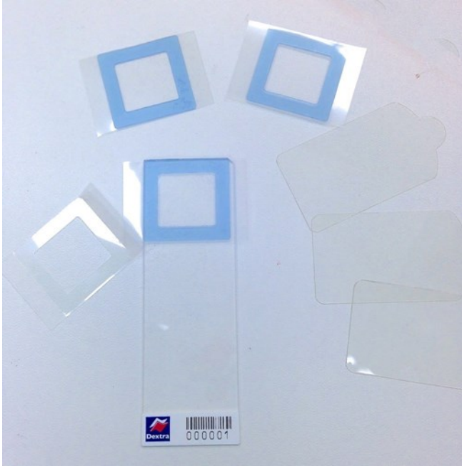
Figure 1b: Positioning of the top of the Gene Frame on the Glycan Array Kit slide.
