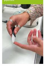
D. The glass transfer pipette is then connected to a Tygon® tube with a blue tip at one end a yellow one at the other end to hold it (then, indeed it is on you to decidal)
